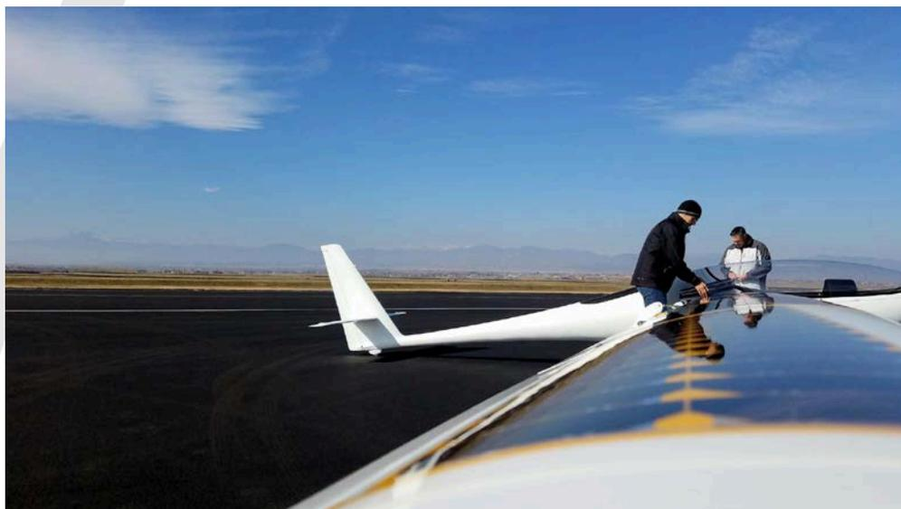
Bye Aerospace StratoAirNet with Integrated Wings Populated with SolAero Solar Cells
